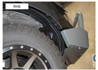
23. Align the bull bar to vehicle so that the guard clearance is 20 to 25 mm, and wing is aligned with wheel arch, then tighten all bolts.
