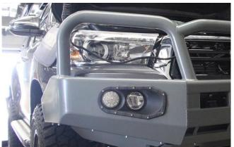
28. Fit plastic lamp housing to bull bar and secure it using :
