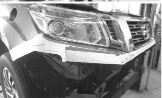
8. Trim bumper as marked, de-burr and clean edges and refit to vehicle using original fasteners in remaining positions.
