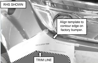
2. Cut out templates supplied, and attach it to bumper, then mark trim line on template as shown.
