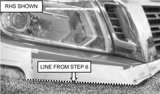
6. Mark a straight line from trimmed corner template to end of the previous marked line.
