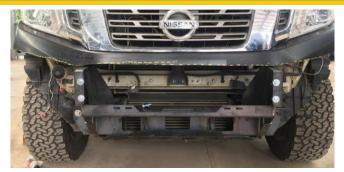
16. Install winch frame (bar mount) on the vehicle chassis rail ends using original bolts from intrusion beam. Centralise and tighten in place.
