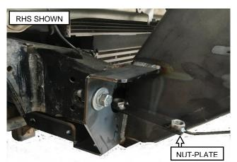
17. Insert the inner chassis nut-plate (M12) into the RHS Chassis through the chassis rail end plate, ensuring the M12 nuts of the nut-plate is positioned towards the top of the vehicle & position it over the two holes located in the underside of the chassis rail.
