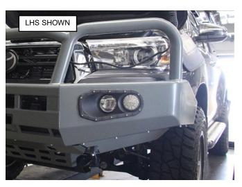
15. Install lamps to bullbar. Indicator from front and fog light (optional) from rear using supplied fasteners. Patch Indicator/park wiring into vehicle lamp wiring loom. Plug in foglamps if installed. Check all lights operate correctly.
