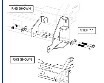
8. Install winch frame (bar mount) on the vehicle chassis rail ends, centralize, then tighten it in place, using original bolts from intrusion beam in original position as indicated.
