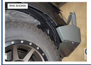
13. Align the bull bar to vehicle so that the guard clearance is 20 to 25 mm, and wing is aligned with wheel arch, then tighten all bolts.
