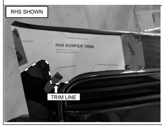
6. Cut out templates supplied, and attach it to bumper, then mark trim line as shown.
