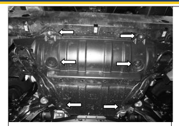
14. Remove and retain the steering guard from vehicle, retaining the fasteners (6) as shown for re-use.
