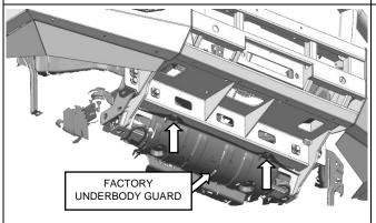
37. Refit the factory underbody guard to its original position, securing it at the rear with original fasteners, except for the indicated position securing it to the bar mount.
