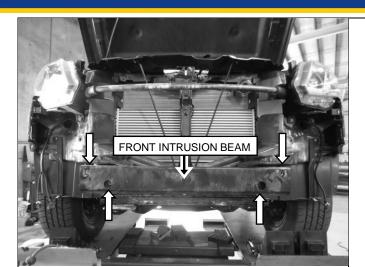
18. Remove and discard the front intrusion beam and the indicated fasteners (4).
