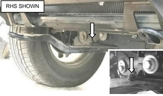
17. Loosen, but don't remove the indicated fasteners, so as to allow the front of the tow points to drop slightly.
