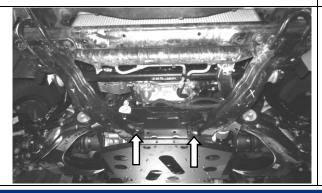
35. Tighten the OE fasteners loosened in steps 16 & 17.
