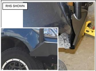
29. Align the bull bar to vehicle so that the guard clearance is 20 to 25 mm, and wing is aligned with wheel arch, then tighten all bolts.
