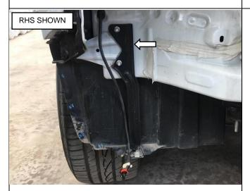
20. Remove and discard the associated bracket from both sides of the vehicle.
