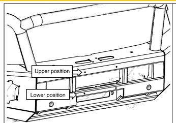
39. Fit the number plate to bull bar in upper or lower mounting position. Optional hinged mount can also be used as shown in next.
