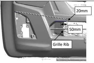
10. Mark a line from the end of the previous line to a point approximately 50mm inboard of the outer grille rib and 20mm up. Drop line down to bumper opening.
