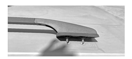
9. From inside the canopy, install & lightly tighten using flat, spring washer & nut.
