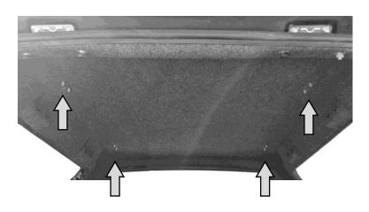
10. Check roof rail position & adjust if required, prior to tighten to **6Nm.**
