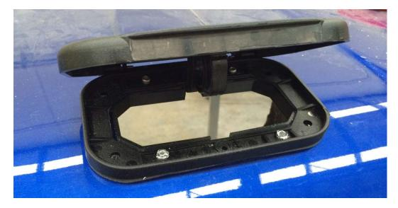
A new base plate has been designed to fit vents to Flexisport, FlexiXover & FlexiTrade canopies
