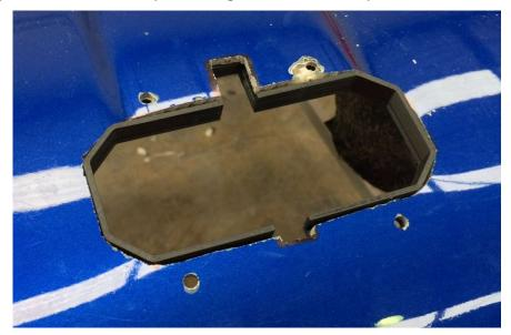
3 Also use the backing plate as a guide to drill the mounting holes through the thick foam and vent base (non standard hole positions) - be careful not to drill through the vent upper flap!. The foam seal may need square notches cut by hand to match the cutout shape and ensure clearance to the vent moving parts
