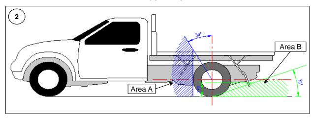
As can be seen in **Diagram 2** the outlines of areas A & B enclose the area that must be covered to be legally compliant. The area to the front of the wheel is obviously covered by the tray and the cab while more attention will need to be paid to the rear to ensure compliance.
