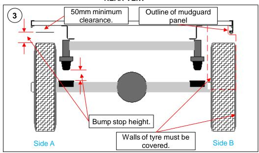
Mudguards must be fitted so that the walls of the tyre, measured at the top of the wheel, (ie away from the bulge at the bottom) are covered by the outer extremities of the guard including any mudflap fitted.
