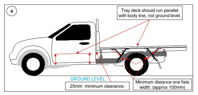
When veiwed from the side a utility vehicle will be found to sit higher at the rear than the front, this is done to allow for load carrying to compress the springs. See **Diagram 4.**
