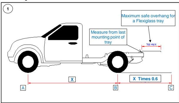
In **Diagram 1** A and B are the wheel centerlines, ie the "wheelbase" of the vehicle. B-C represents the maximum legaly allowable rear overhang for that particular vehicle which is always 60% of the wheelbase.
