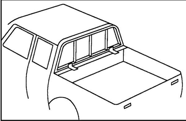
1. Remove the existing Header bar from the front of the tub using a T40 Torx screw bit, remove the 3 screws on each of the inside sections and 5 across the top of the header bar. Remove the Header bar.
